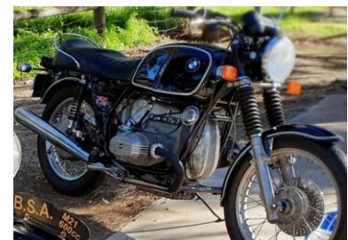
The 750cc engine was used up until 1979 and although there were faster bikes in BMW's line up, this mid-sized unit was often cited as the best compromise between power and smoothness. Being a /7 model this bike benefited from the latest improvements developed from the larger bikes and the result was a fine performing bike with an under stressed engine, able to provide years of reliable biking. The BMW R75/7 Claimed by some traditionalists to be the best BMW twin ever. A late 750 BMW is a good choice for anyone seeking long term ownership of a classic BMW twin.
